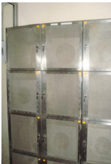
Arthropod cages constitute the primary containment in insectariums. Adult mosquitoes kept in rearing cages. Access is via a 60cm long cloth sleeve (surgical stockinet) that fits an opening on 1 side of the cage. The cages are kept in ventilated secure cabinets. (Source: IMR)
