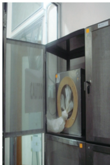
Arthropod cages constitute the primary containment in insectariums. Adult mosquitoes kept in rearing cages. Access is via a 60cm long cloth sleeve (surgical stockinet) that fits an opening on 1 side of the cage. The cages are kept in ventilated secure cabinets. (Source: IMR)
